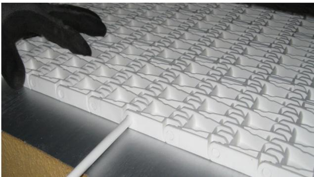
During the life-time of the drying installation, there is a real chance that a larger item (e.g. a rock, a screw driver, a piece of wood or metal) is accidentally put onto the drying belt which damages the belt. Just imagine what would happen with a non-modular belt...
